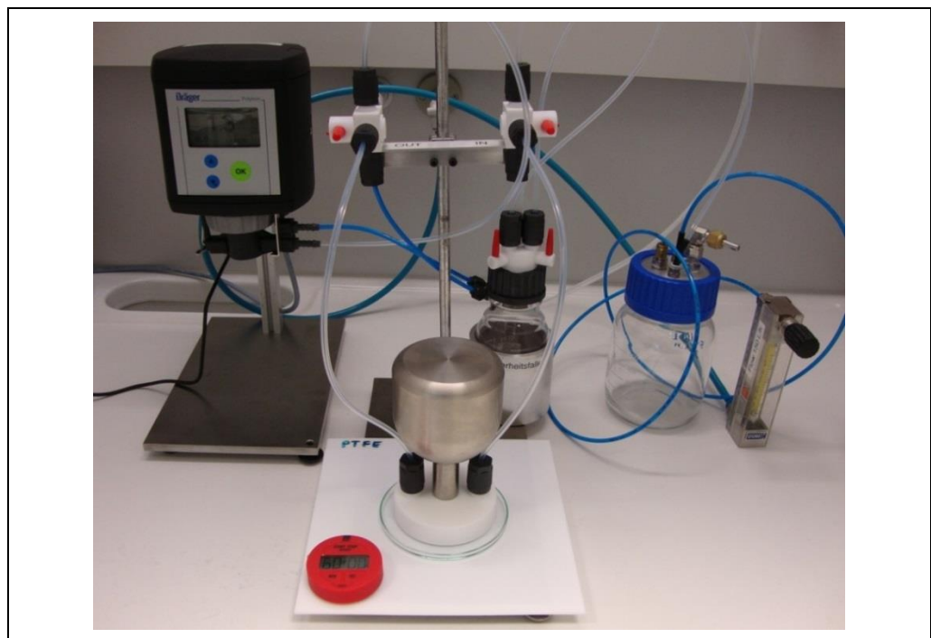
Figure 71 Experimental design. Left: H 2 O 2 measurement device; center: exposure chamber, right: H 2 O 2 source
