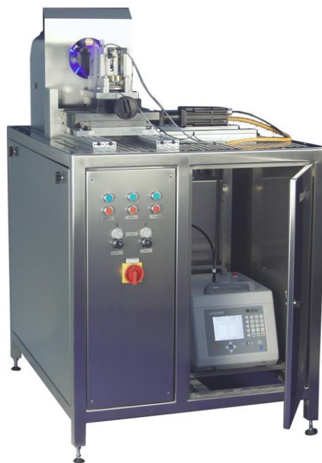
Figure 4 Cleanroom-suitable material test bench "Material Inspec" developed by Fraunhofer IPA with module for ball on disk test. The module can be replaced if necessary with the module for reel on disc test.
